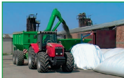
The harvested grain will be stored in a silage bag by using the Farm Bagger
